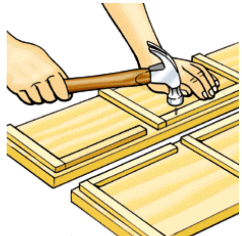
Fig. 6 Nail and glue shelf cleats and back cleats to the side panels. Note that cleats are recessed 3/8 in. from back edge of sides.
