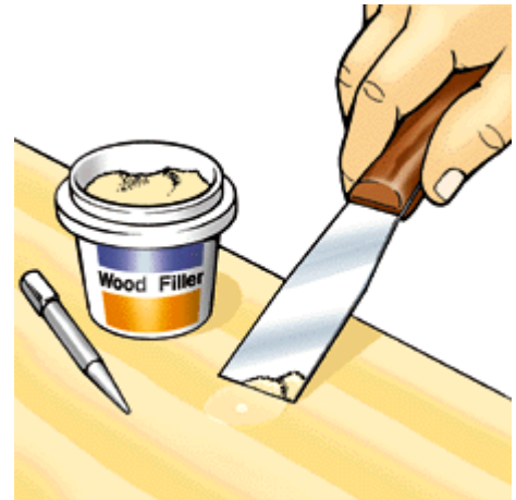
Fig. 11 Use a nail set to drive all nails below the surface. Then apply wood filler over the nailheads with a putty knife.
