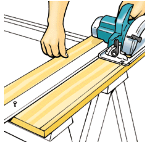
Fig. 3 Use a straight strip as a guide when ripping stock for the four lower shelves to 8 \frac{7}{8} in. The top shelf remains a full 1 x 10.
