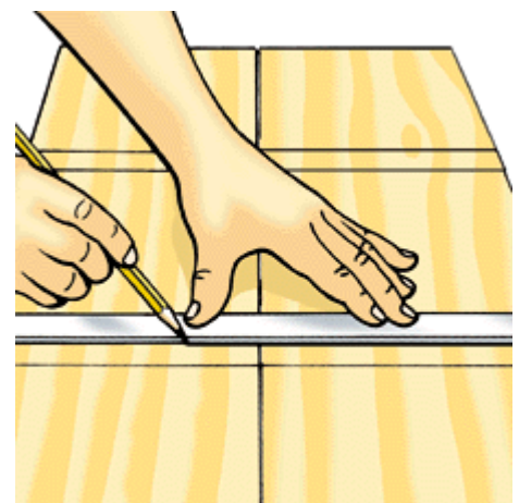
Fig. 5 Butt sides together with shelf-location marks on outer edges. Use a straightedge to extend the shelf marks
