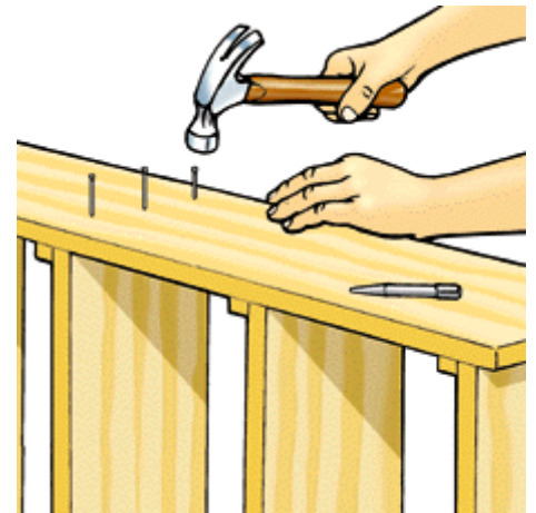
Fig. 7 Secure one side to the shelves with glue and 6d finishing nails. Then flip the assembly over and attach the other side. Set all nails.
